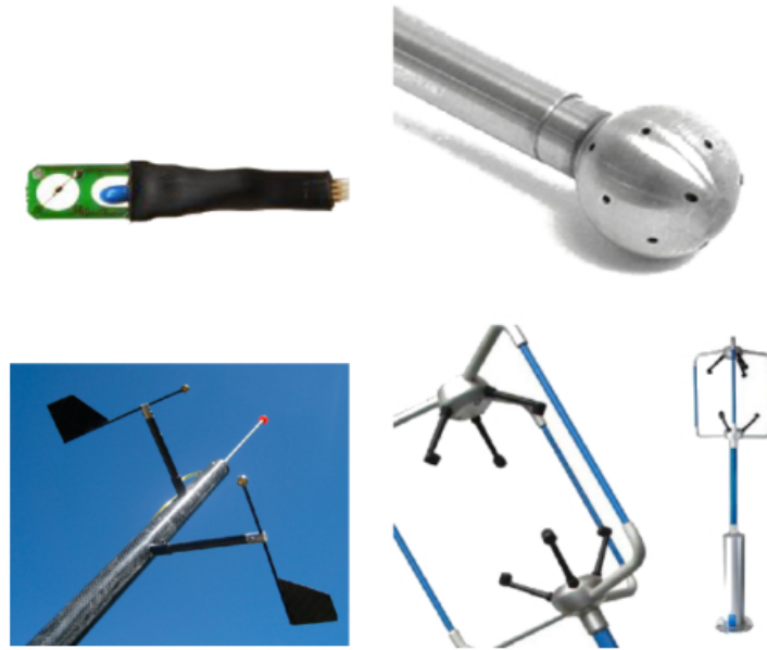
Figure 2.2: Relative Wind Sensors. Clockwise from upper-left: hot wire anemometer, multi-hole probe, sonic anemometer, Pitot probe with vanes
